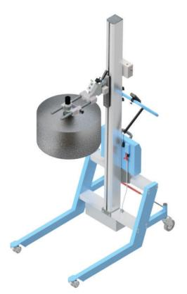
Our Electric Expand-O-Turn™ is an electrically operated core expander for paper and film rolls with 3" and 6" cores and allows for manually rotating the roll. Rolls of varying dimensions, weights up to 300-lbs (depending on roll size), can be picked up from the vertical position at floor/pallet level and deposited at random heights in a horizontal position.
