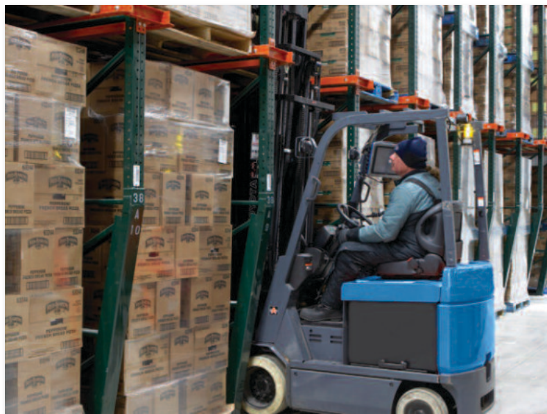
Operator drives directly into the pallet storage lane.
