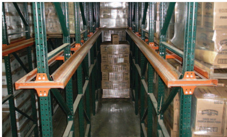
Narrow pallet lanes provide high-density storage.
