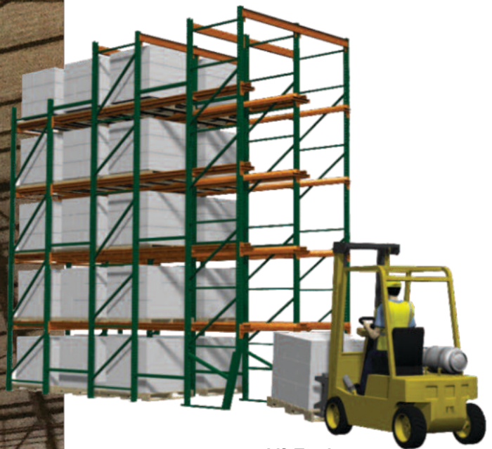
Lift Trucks - Enter the storage system placing the load on the floor or on the pallet rails.
