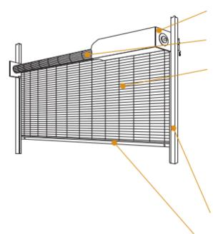
BRACKETS - Steel with SpectraShield® powder coating in Gray.
