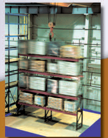
All loads remain intact on racks during the most severe earthquake simulation and structure incurs no damage!
