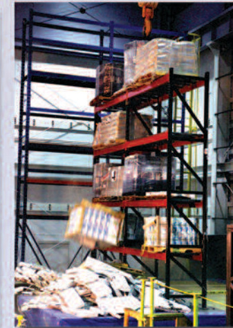
Rack structure continues to shed loads.
