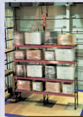
Isolators reduce felt ground forces, loads remain in place.
