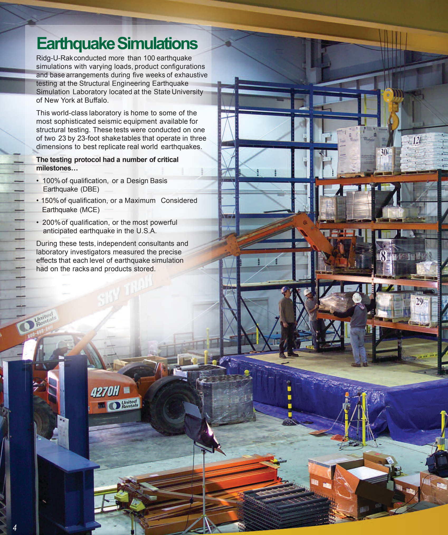
Simulation begins...rack starts to sway, loads start to move.
